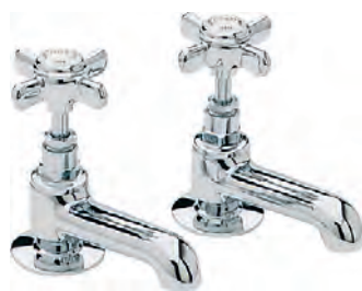
Basin Pillar Taps Spout projection 95mm Full height 120mm Min. operating pressure 0.1bar Valve: Quarter turn ceramic disc
