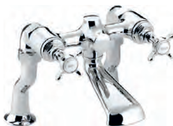
Bath Filler Spout projection 247mm Full height 200mm Min. operating pressure 0.1bar Valve: Quarter turn ceramic disc Inlet centre 100-200mm
