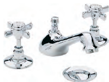
3 Taphole Basin Mixer Spout projection 130mm Full height 100mm Min. operating pressure 0.2bar Valve: Quarter turn ceramic disc
