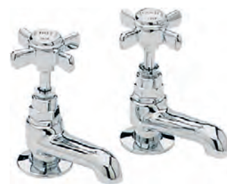
Short Nose Basin Pillar Taps Spout projection 64mm Full height 115mm Min. operating pressure 0.1bar Valve: Quarter turn ceramic disc
