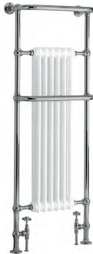
Cabot Height 1500mm Width 580mm Valve centres 350mm Wall to valve centre 105mm Output 2153 Btu (631 watts)
