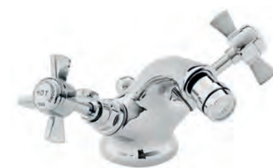
Bidet Mixer Spout projection 110mm Full height 100mm Min. operating pressure 0.2bar Valve: Quarter turn ceramic disc
